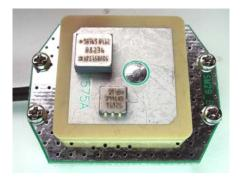
Figure 2 – GPS patch antenna with MEMS yaw-rate linear acceleration sensors.
