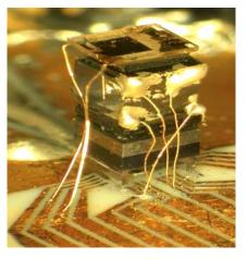
Figure 4 – Chip-scale atomic Cs clock as developed by NIST.
